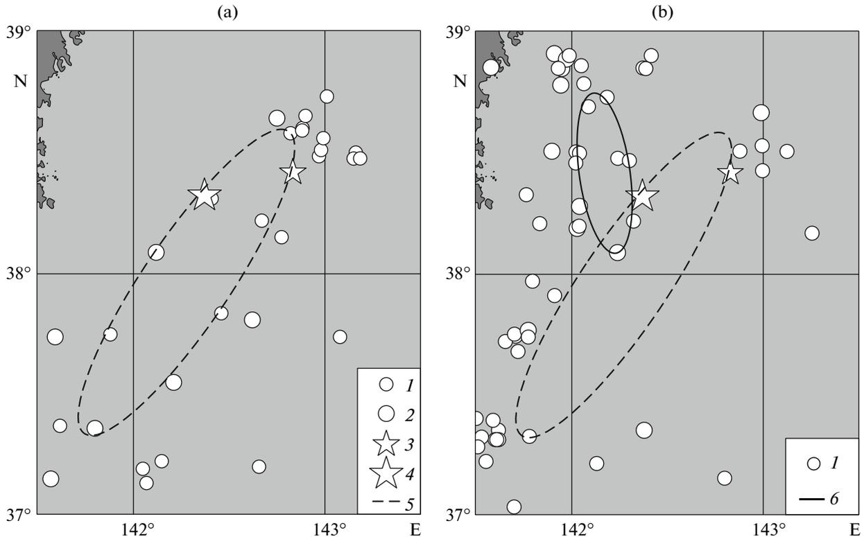
**Fig. 3.** Annular seismicity structures prior to the March 11, 2011, earthquake: (a) for the depth range of 0–33 km: 1,  $5.8 \leq M < 6.5$ , 2,  $M \geq 6.5$ , 3, epicenter of the March 9, 2011, foreshock, 4, epicenter with  $M_w = 9.0$  earthquake, 5, shallow ring, 6, deep ring; (b) for the depth range of 34–70 km: 1,  $5.3 \leq M < 6.5$ , 2, deep ring (the remaining arbitrary notations are the same as in Fig. 3a).
